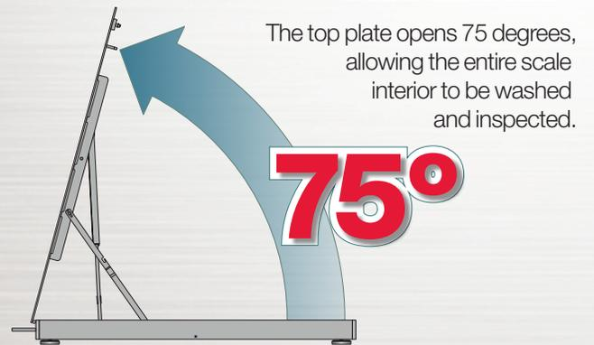
The top plate opens 75 degrees, allowing the entire scale interior to be washed and inspected.
